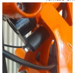
To adjust the steering drift, loosen the screw with a #13 hex key, adjust the steering and tighten the screw. Make sure that the screws are well tightened and that the rubber is intact. Periodically check the state of wear of the steering rubber and if necessary replace it with one of the same type.
